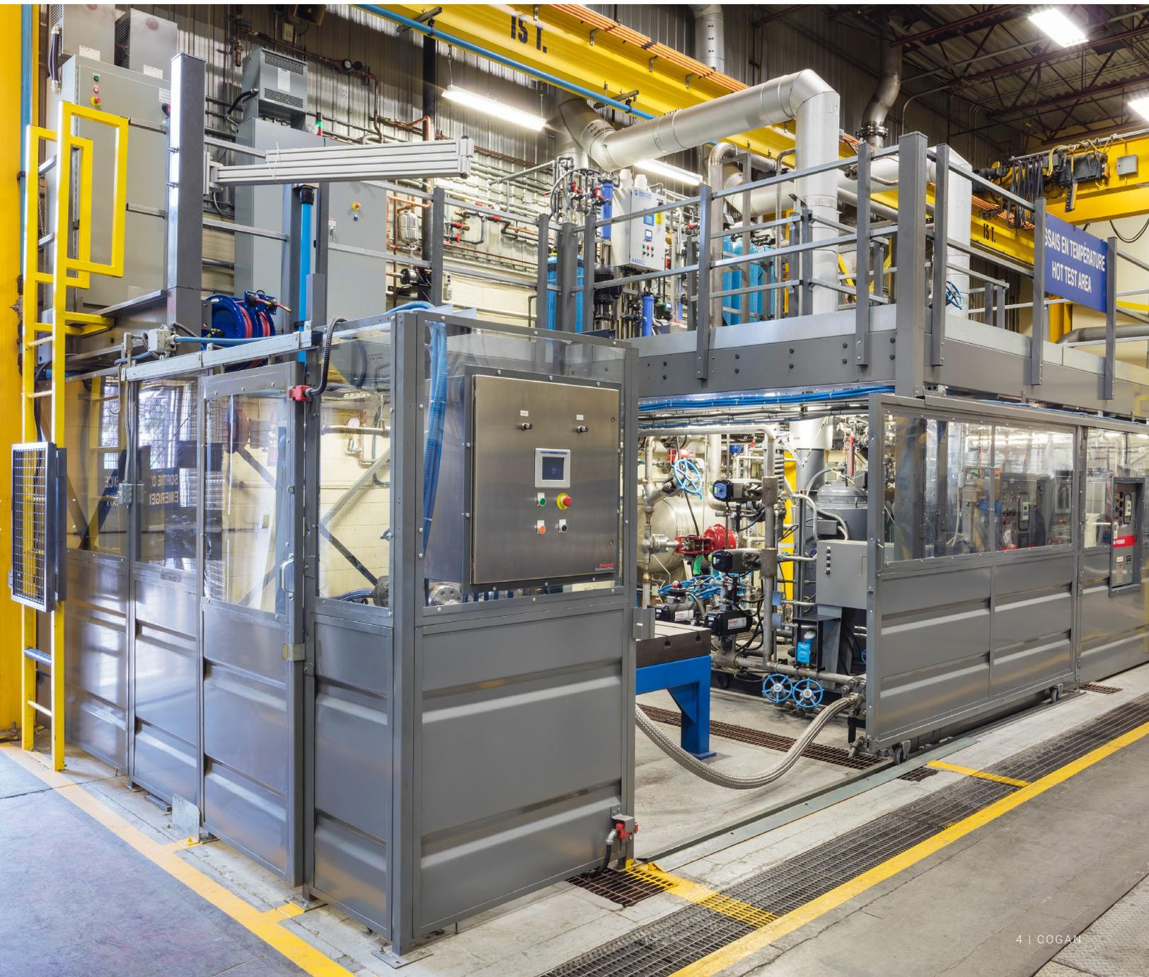
Secure and separate conveyor systems and moving machinery from warehouse traffic with Cogan conveyor guard partitions.
